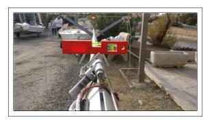
Put your mast horizontal and check it with a bubble level. After this you must be sure that your spreaders are symmetrically opened so put a thin rope to close the spreaders and put on it a bubble level.
